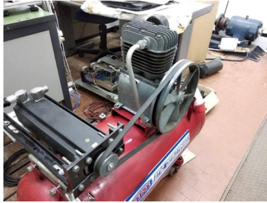
Fig. 18 Air compressor test bench, 9.5 Nm
