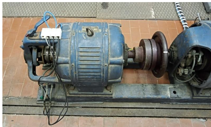
Fig. 114 Induction motor used as EESM
