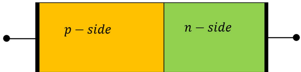
Fig. 8 Rectangular PN junction
