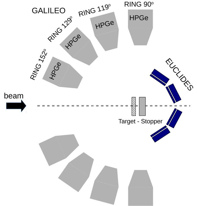
FIG. 2. Schematic view of the GALILEO  $\gamma$ -ray spectrometer coupled to 15 forward-most  $\Delta E$ - $E$  telescopes of EUCLIDES. The target and stopper, installed at the center of the reaction chamber, are schematically illustrated. See text for more details.
