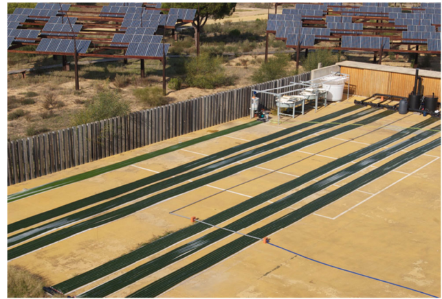
Fig. 2 The two out-door photobioreactors on the 27 Nov 2011. In front, the 6 lanes belonging to the 6 m 3 reactor; in the back, the single lane of the 600 L reactor, used for producing starter culture for the 6 m 3 reactor. The tube crossing the 3 front lanes is the harvest line
