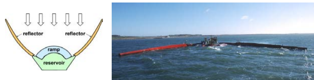
Figure 30. Views of the small-scale Wave Dragon (left) (Reproduced with permission 5139270373963 from [32], Elsevier, 2010) and its working principle (right) (Reproduced with permission 5139270591282 from [99], Elsevier, 2009).
