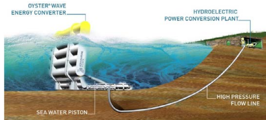
Figure 25. Working principle of Oyster [86,87].
