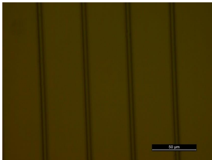
Figure 33 : Optical microscope image of 3.9 \mu\text{m} lines created using photolithography on Si intended to be 2 \mu\text{m} using SF11/S1813 bilayer exposed for 5 s and developed for 30 s. Reduction in development time required as more control of the development rate than exposure. Black line edge of photoresist.
