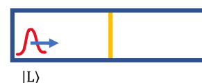
Fig. 1 The set-up. A spin 1/2 particle in a box with a completely reflective wall on the left, a spin-independent, partially transparent partition in the middle with, very small transmissivity, and a spin-dependent wall on the right, which is totally reflective for spin |\uparrow_z\rangle and totally transparent for |\downarrow_z\rangle . The particle starts in a wavepacket |L\rangle , next to the left wall, moving right and with spin |\uparrow_z\rangle .
