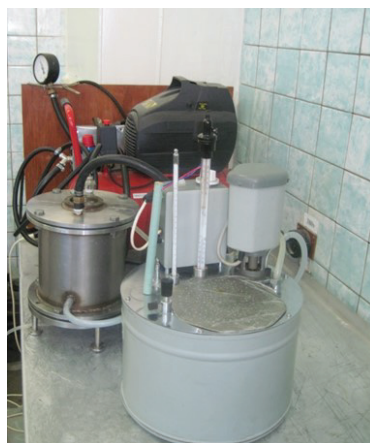
Fig. 2. Experimental membrane plant for concentrating low-fat dairy raw materials
