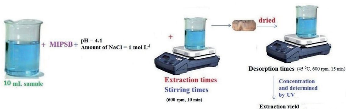
Figure 7. Schematic of MIP-coated SBSE for naphthalene sulfonates. Reprinted by kind permission from Ref. [52]. Copyright 2018 Taylor and Francis.
