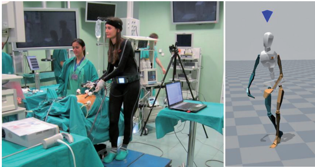
Figure 3. Motion tracking system based on inertial sensors placed on the surgeon's body (left). A biomechanical model of the subject is created in real time (right). (Source: [17]).
