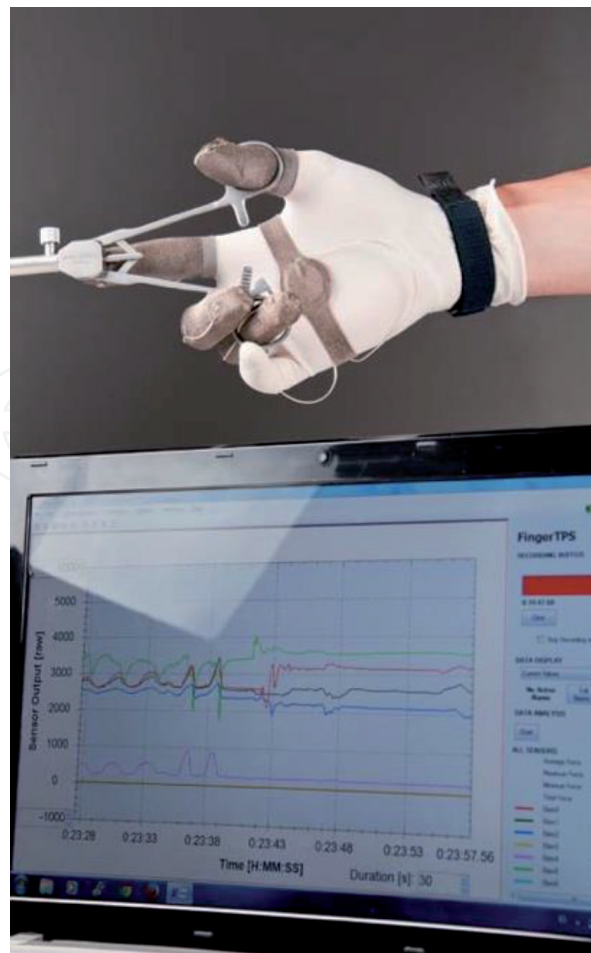
Figure 5. Use of the FingerTPS™ system during the handling of laparoscopic instruments with a ring handle. (Source: [3]).
