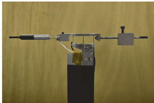
Figure 2. View of the sting balance two modules, drag and lift.
