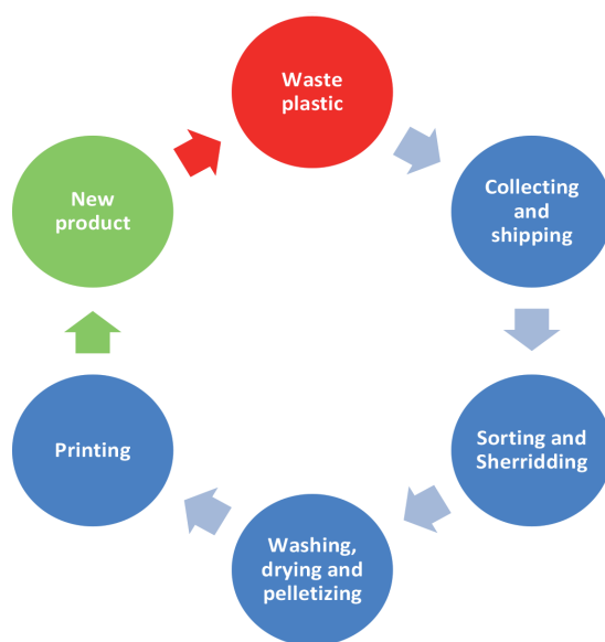
Figure 1. Pathway to recycle thermoplastic materials.
