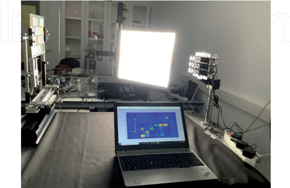
Figure 12. Hyperspectral CCD calibration procedure.
