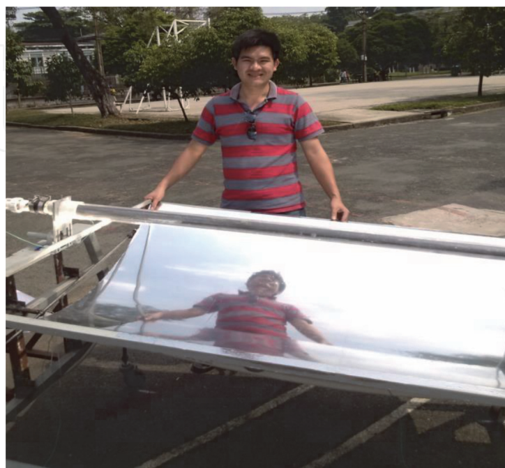
Figure 2. The parabolic trough solar collector being tested at the Ho Chi Minh City University of Technology.
