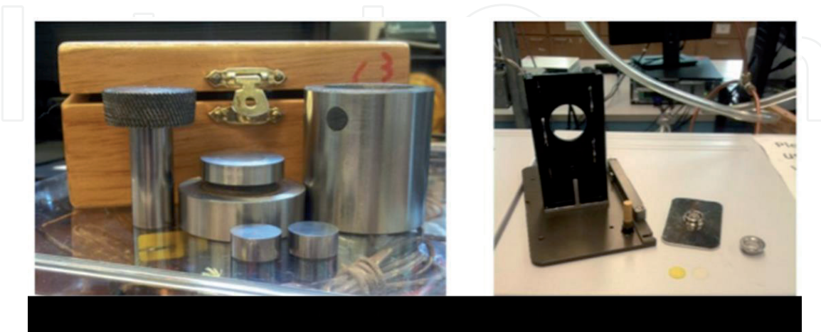
Figure 12. Typical setup of FTIR for sample preparation for both traditional and modern methods [47].
