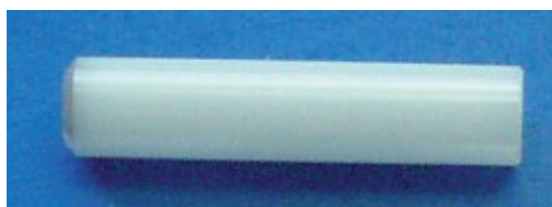
Figure 11. A general torlon based rotor was used for ^{29}\text{Si} solid-state NMR technique [38].
