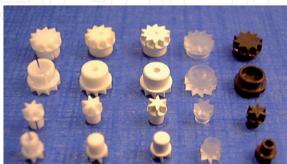
Figure 8. Type of caps used for rotors (typical materials used ZrO 2 , Macor, KeI and Vespel) [40].
