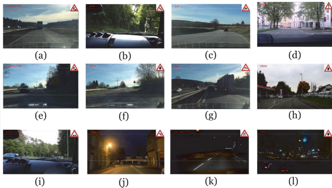
Figure 37. The overall results for triangular speed regulatory road signs detection (a-c) during the daytime, (d-g) during the backlight condition, (h-i) during the cloudy weather (j-l) during the night.
