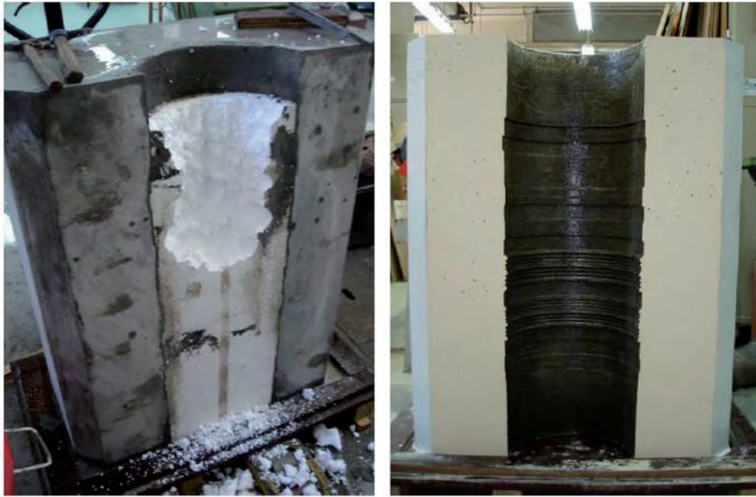
Figure 4. Removing of polystyrene core (left); final shape of the setup with varying roughness and hole diameter (right).
