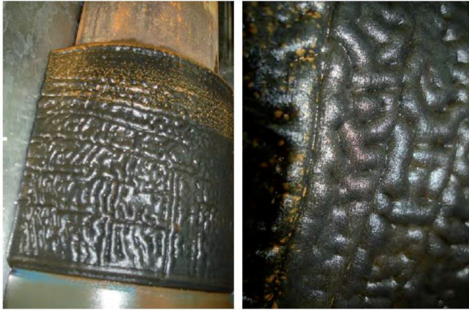
Figure 17. Pictures of the elastomer surface that swells against formation (concrete block), after swelling and partial de-swelling.
