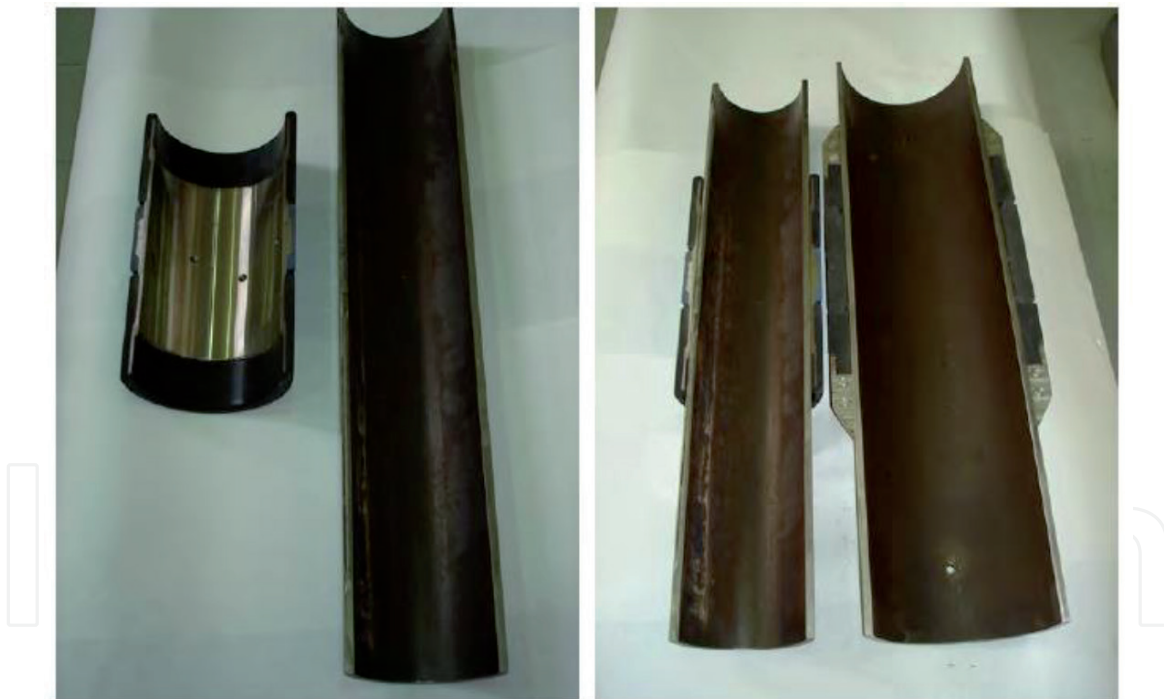
Figure 7. Half portions of inside swell packer and pipe (left); inside and outside swell packers fitted on respective pipes (right).
