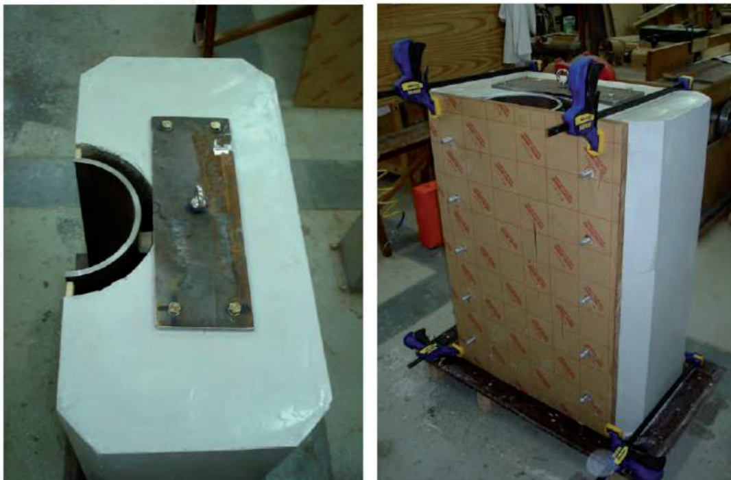
Figure 9. Assembled setup with inner and outer packers, plexi-glass front and top walls, and lifting arrangement.
