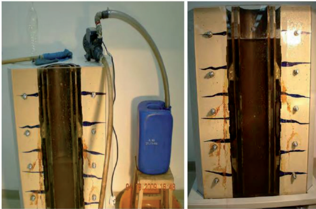
Figure 11. Flushing and cleaning of the unit (left); water fill-up after flushing (right).
