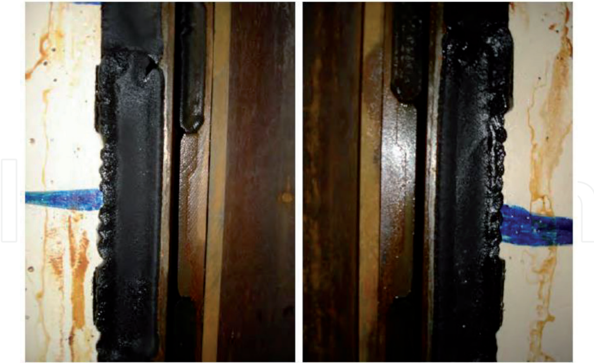
Figure 13. Near-complete swelling of the outer elastomer seals against cavities of varying diameter and roughness.
