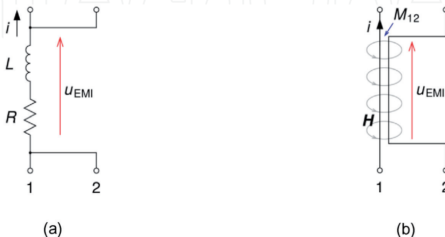
Figure 5. Equivalent circuit: Galvanic coupling (a) and inductive coupling (b); R – Resistance, L – Self-inductance, M_{12} – Mutual inductance between wires, i – Disturbing current, u_{\text{EMI}} – Disturbing voltage, H – Magnetic field strength.
