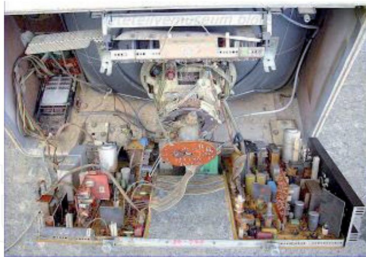
Figure 3. Digital TV receiver contains Mn-ferrites deflection yokes [15].
