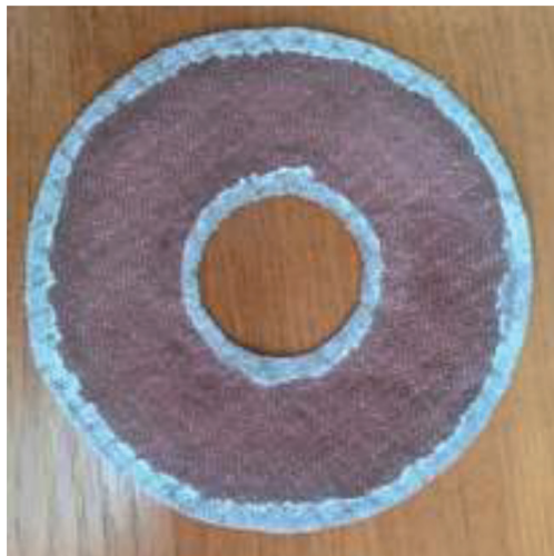
Figure 4. Same woven fabric with plasma copper coating.
