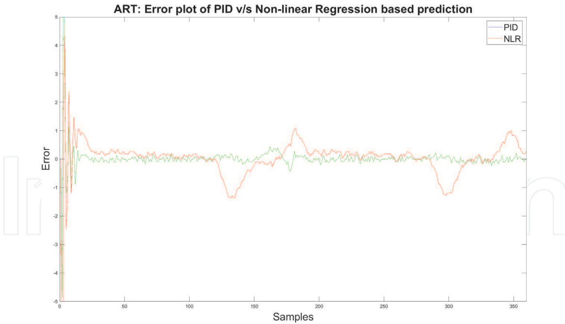
Figure 4. Error plots of comparison of prediction performance by PID and ANN-NLR algorithms for arterial pressure.
