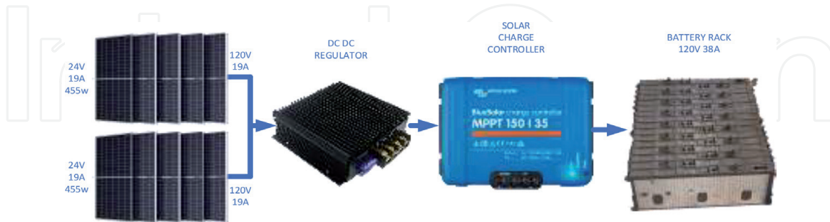
Figure 15. Components of the solar powered charging unit.
