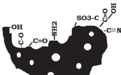
Figure 4. Model of various organic functional groups on the activated carbon [30] (● = carbon matrix; ○ = pores).
