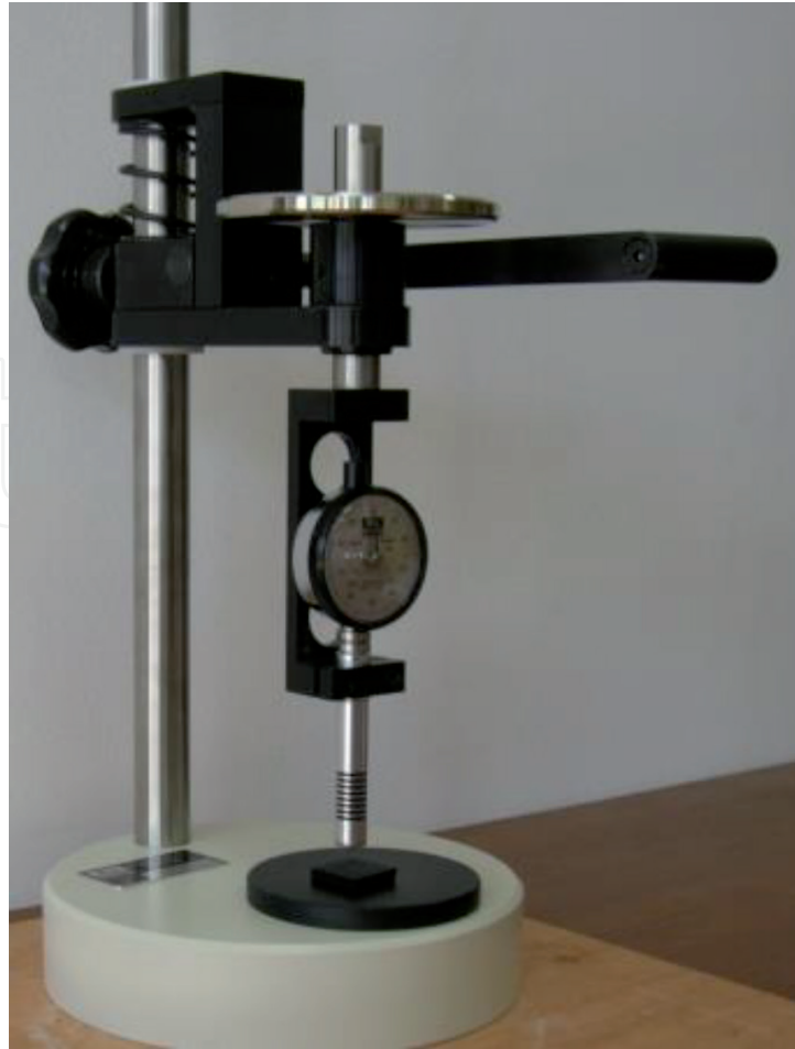
Figure 3. Durometer for hardness testing.
