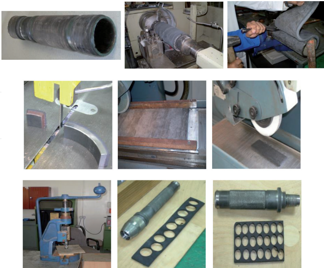
Figure 2. Different stages in sample preparation: Cutting sections from packer, and plate samples from sections; removing elastomer from pipe; surface grinding; cutting discs and rings using die-and-punch set.
