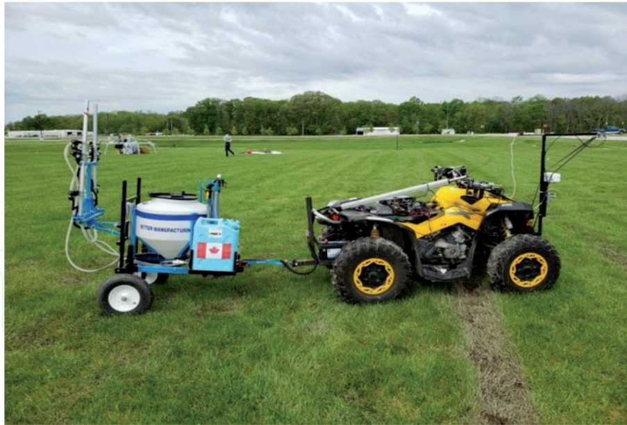
Figure 13. CanAm ATV and setter plot sprayer used by a group of undergraduate University of Manitoba students to produce an autonomous sprayer for the agBOT challenge in 2019.
