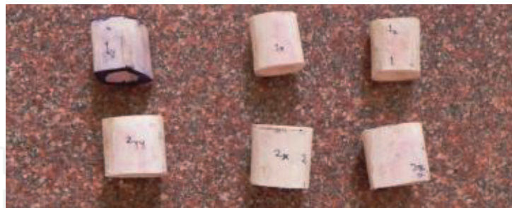
Figure 2. Test sample, cubes of water Buffalo female ( Bubalus bubalis ), cut out of test specimen.
