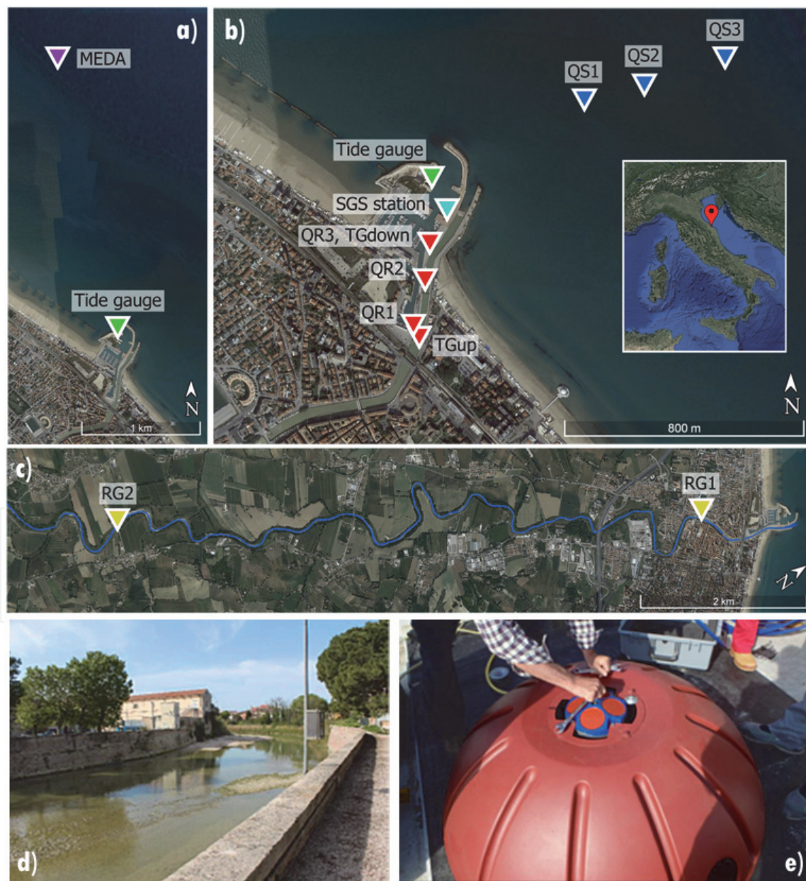
Figure 1. Instrumentation employed for the MR monitoring: a) locations of the ADCP and tide gauge in the coastal region; b) locations of sensors displaced within the final reach of the river and the offshore area; c) locations of the two river gauges. Photos illustrating: d) the river portion near the RG1 instrument; e) the ADCP deployed at the MEDA station.
