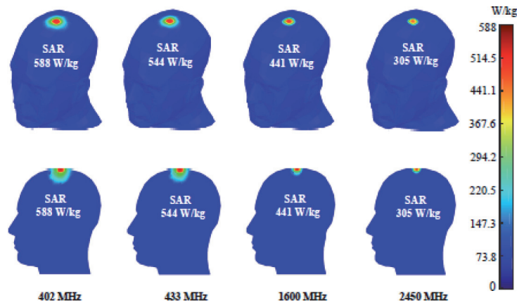
Figure 18. Simulated averaged SAR surface (top row) and coronal (bottom row) distributions over 1-g of tissue in an anatomical human head model [37].
