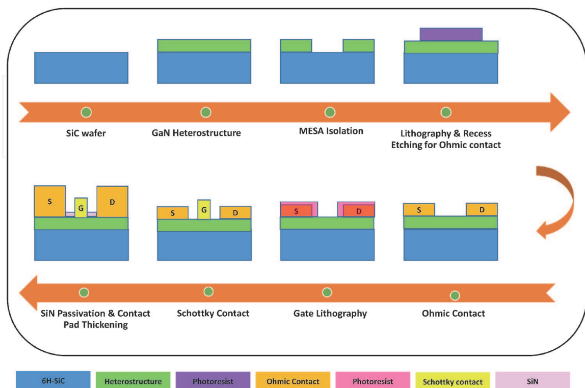
Figure 14. GaN HEMT fabrication flow along with the cross-sectional view of the device.
