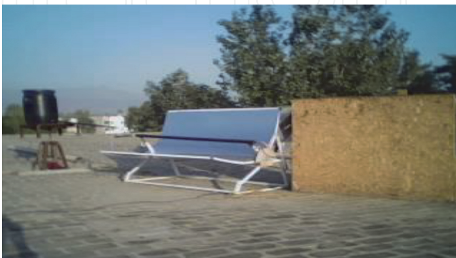
Figure 3. General view of parabolic trough solar water distillation unit.
