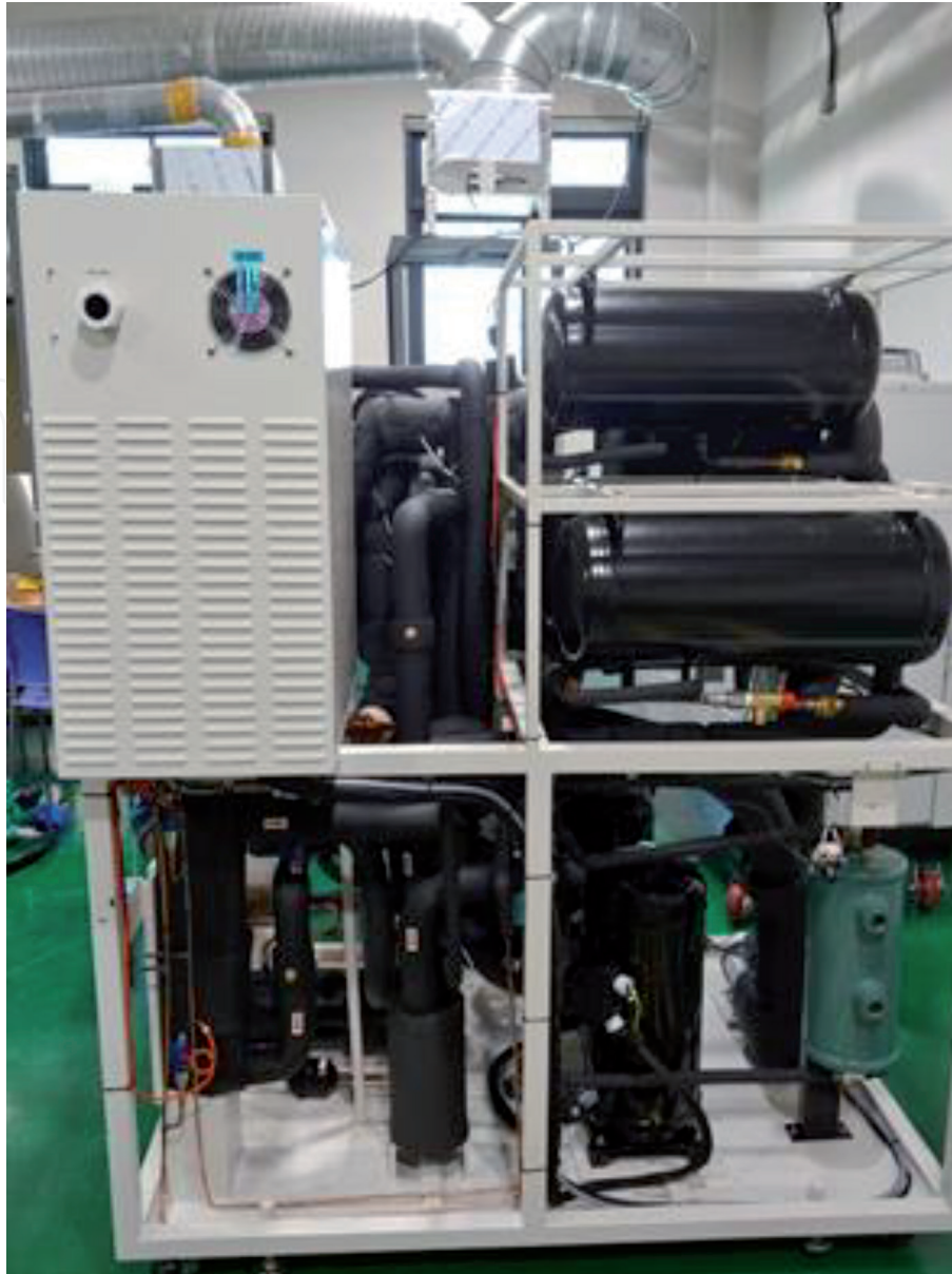
Figure 10. Experimental device of cascade MR refrigerator.
