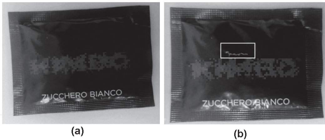
Figure 9. Sugar bags. (a) Standard packaging. (b) Defect packaging highlighted in the box.
