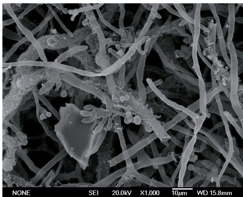
Figure 3. SEM image of the fungus Aspergillus niger grown on fluorescent lamp powder.
