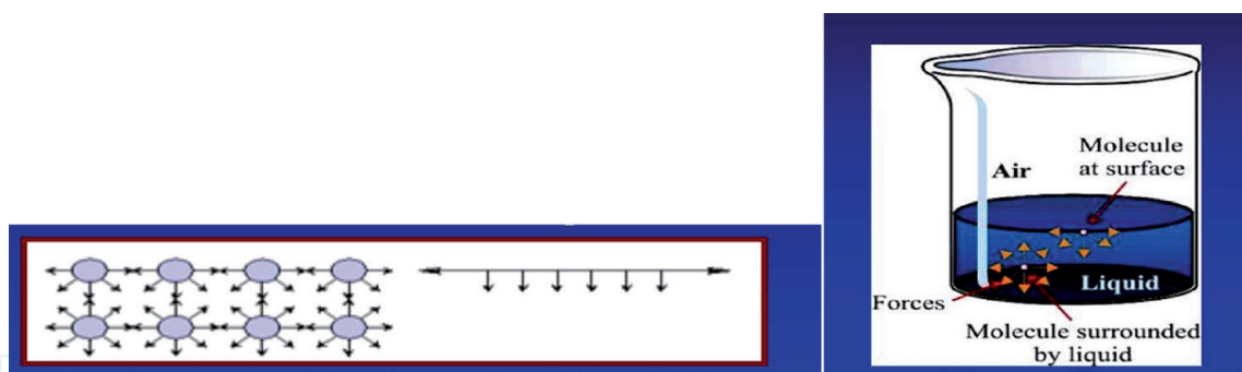
Figure 3. Surface and Interfacial tensions for the molecules in bulk liquid.
