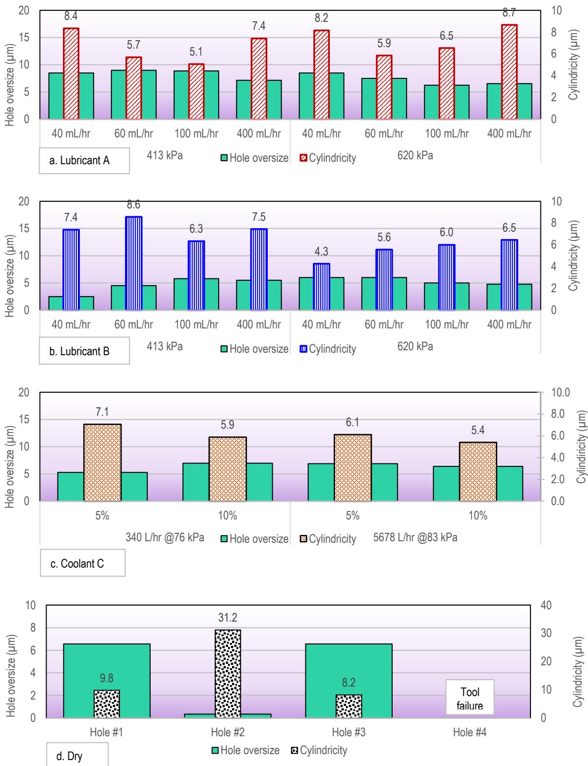
Figure 13. Average hole oversize and cylindricity of drilled holes.
