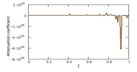
**Figure 8**. Variation of attenuation coefficient of Stoneley waves with respect to  $\xi$  when  $a_1=0=a_3$
