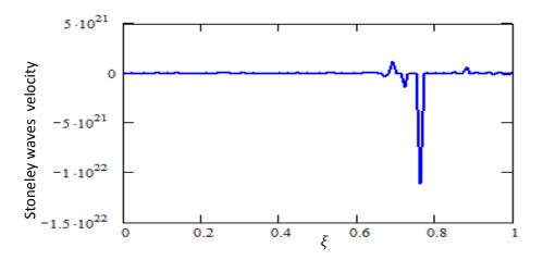
**Figure 4** .Variation of Stoneley waves velocity with respect to  $\xi$  when a<sub>1</sub>=0.03,a<sub>3</sub>=0.06.
