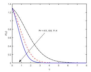
**Figure 14.** Temperature distribution for different values of Pr
