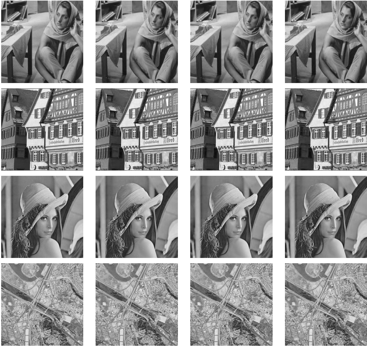
Figure 10. Test images and compression results. Top to bottom: barbara, house, lenna, and sandiego. Left to right: original, CDF 9/7 with SPIHT (Said and Pearlman, 1996) at 0.5 bpp, BFB 11/9 EP3 with SPIHT at 0.5 bpp, and BFB 15/13 EP3 with SPIHT at 0.5 bpp
