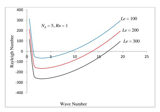
**Figure 2**. Variation of stationary Rayleigh number *Ra* with wave number *a* for different values of Lewis number *Le*
