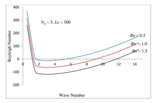
**Figure 3.** Variation of stationary Rayleigh number Ra with wave number a for different values concentration Rayleigh number Rn
