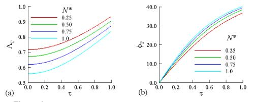
**Figure 6.** Amplitude and phase of surface heat transfer showing the effect of  $N^*$  when  $\varepsilon = 0.1$ , Pr = 9.0,  $N^* = 1.0$
