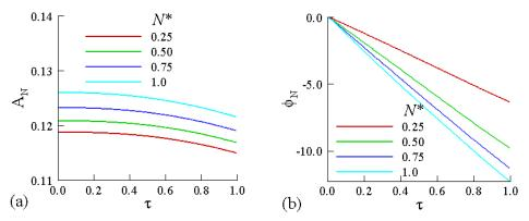
**Figure 7.** Amplitude and phase of couple stress showing the effect of  $N^*$  when  $\varepsilon = 0.1$ ,  $Pr = 9.0, N^* = 1.0$
