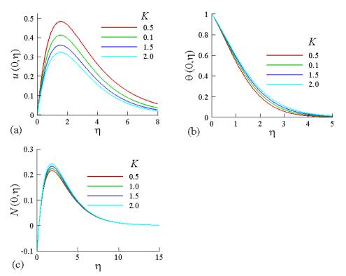
**Figure 11.** Numerical values of (a) velocity profiles (b) temperature profiles and (c) angular velocity profiles for different values of K against  $\eta$  while Pr = 9.0 and  $\omega = 1$
