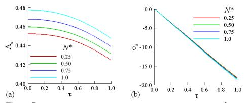
**Figure 5.** Amplitude and phase of surface shear stress showing the effect of  $N^*$  when  $\varepsilon = 0.1$ ,  $Pr = 9.0, N^* = 1.0$
