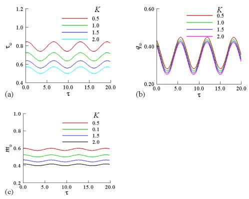
**Figure 9.** Numerical values of (a) shear stress (b) surface heat transfer coefficient and (c) couplestress for different values of K against values of  $\tau$  while Pr = 9.0 and  $\omega = 1$
