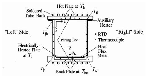
Figure 2. Cubical experimental apparatus with auxiliary heaters
