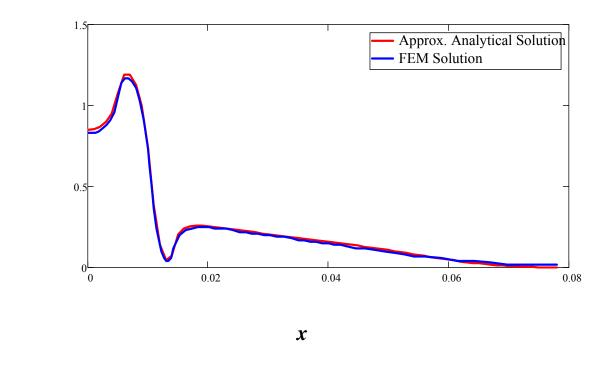
**Figure 7.** Comparison of the relative temperature Distributions, T(X, 0) - T(0.078, 0), along Y = 0 for case #4 With  $\Delta = 2\rho = 0.0641$  (or F = 2g = 5 Mm) based on the approximate analytical solution and the Fem solution
