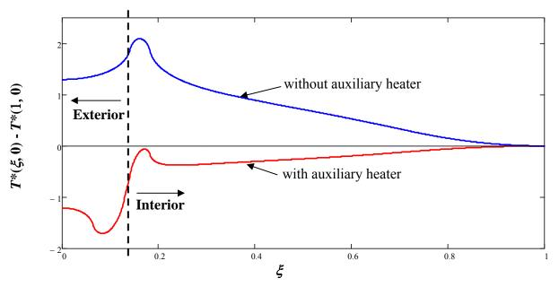
**Figure 8.** Dimensionless relative temperature distributions,  $T^*(\Xi, 0) - T^*(1, 0)$ , along Z = 0 for case #4 with  $\Delta = 2\rho = 0.0641$
