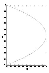
**Figure 1.** Base flow velocity component in the horizontal direction versus z
