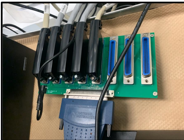
Figure 11. Master PCB is connected to five harmonica adapter using telecom cables. This system can grow to support a total of 96 sensors.
