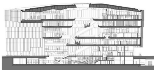
Fig.26: section of the Deichman library showing the folded concrete structure and the tension rods source: arch daily
