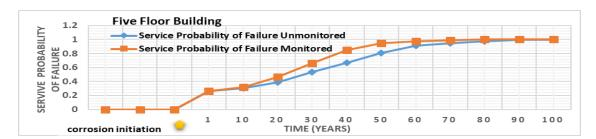
Fig.4: The Service Probability of Failure of the five floor building using both monitored and unmonitored data over 100 years from corrosion initiation.
