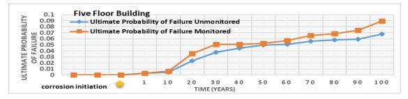
Fig.5: The Ultimate Probability of Failure of the five floor building using both monitored and unmonitored data over 100 years from corrosion initiation
