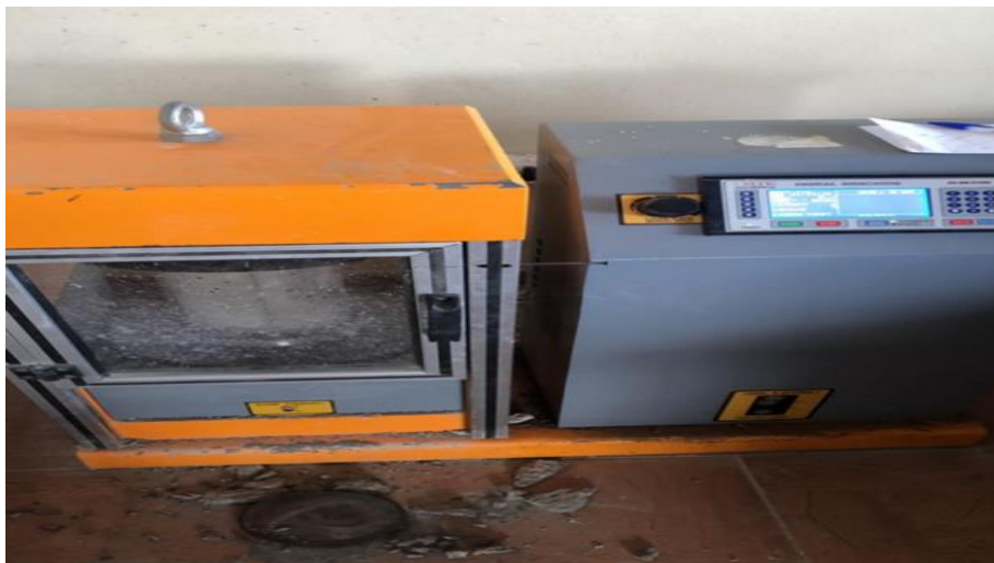
Fig.7: Cylindrical Specimen under Compressive Strength Testing
