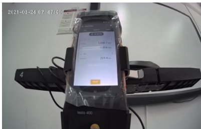
Fig. 2c: Sample of remote measurement taken by the wireless camera connected to the smartphone.
