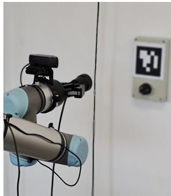
Figure 8. Center gripper taking the fiducial marker as a visual reference.
