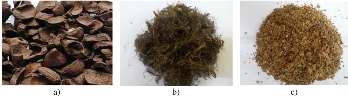
Fig. 1. Palm nut shells a), Palm nut mesocarp fibers b), Coffee husk c).
