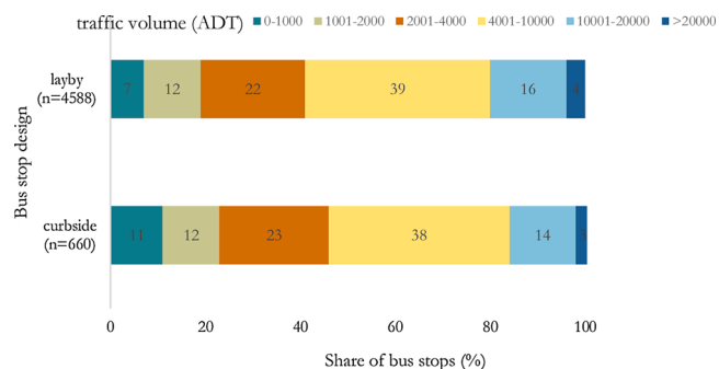
Fig. 7. Distribution of curbside and layby stops on roads with different traffic volumes in built-up areas in Norway, according to data registered in Vegkart.
